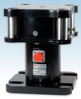
A stainless steel compression load cell housed in an integral mounting assembly, which is ideal for general commercial weighing of large tanks, silos and vessels, particularly in the cement, minerals and coal industries. The design ensures optimum performance and eliminates many traditional problems encountered during the installation of high capacity weighing systems. The T30 load cell and mounting assembly are supplied as a complete locked unit, ready to install.
